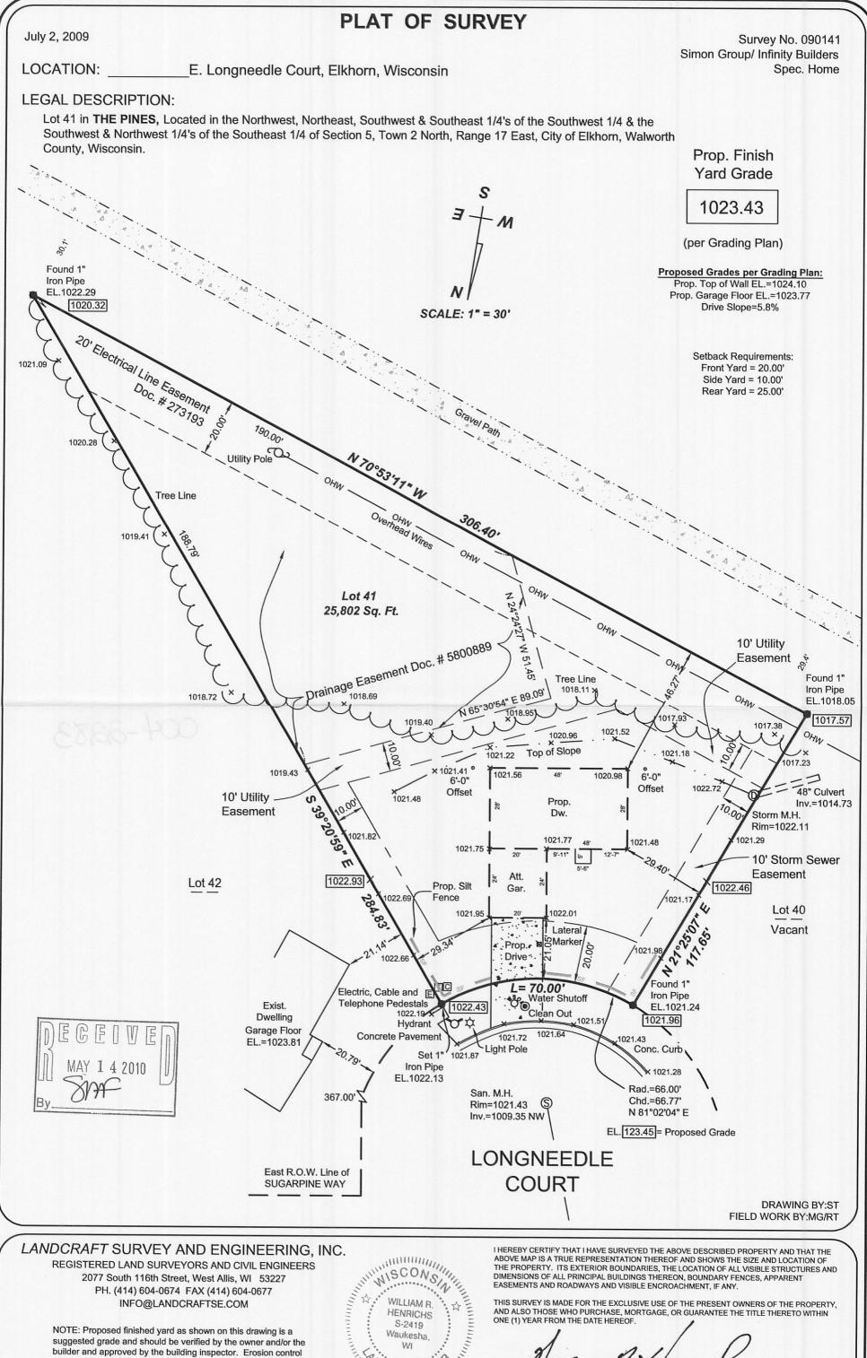
NOTE: Proposed finished yard as shown on this drawing is a suggested grade and should be verified by the owner and/or the builder and approved by the building inspector. Erosion control measures are suggested and must be verified/adjusted by the builder and/or building inspector based on site conditions.
